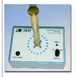
The Comtest Field Reference Source is a stable, broadband reference generator. The source is designed for rapid evaluation of an EM test site and its performance. The field reference source uses a precision transmission line pulser to generate an accurate, stable output at a repetition rate of 1 or 5 MHz.
